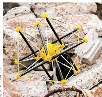
SIX SHOCK ABSORBERS PROTECT THE CORE OF A NEW ROBOT, SO IT CAN SURVIVE FALLS FROM HIGH ALTITUDES.
