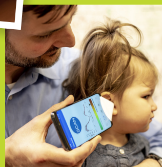
A PHONE APP AND A PAPER CONE REVEALS LIQUID BEHIND THE KID'S EARDRUM.
